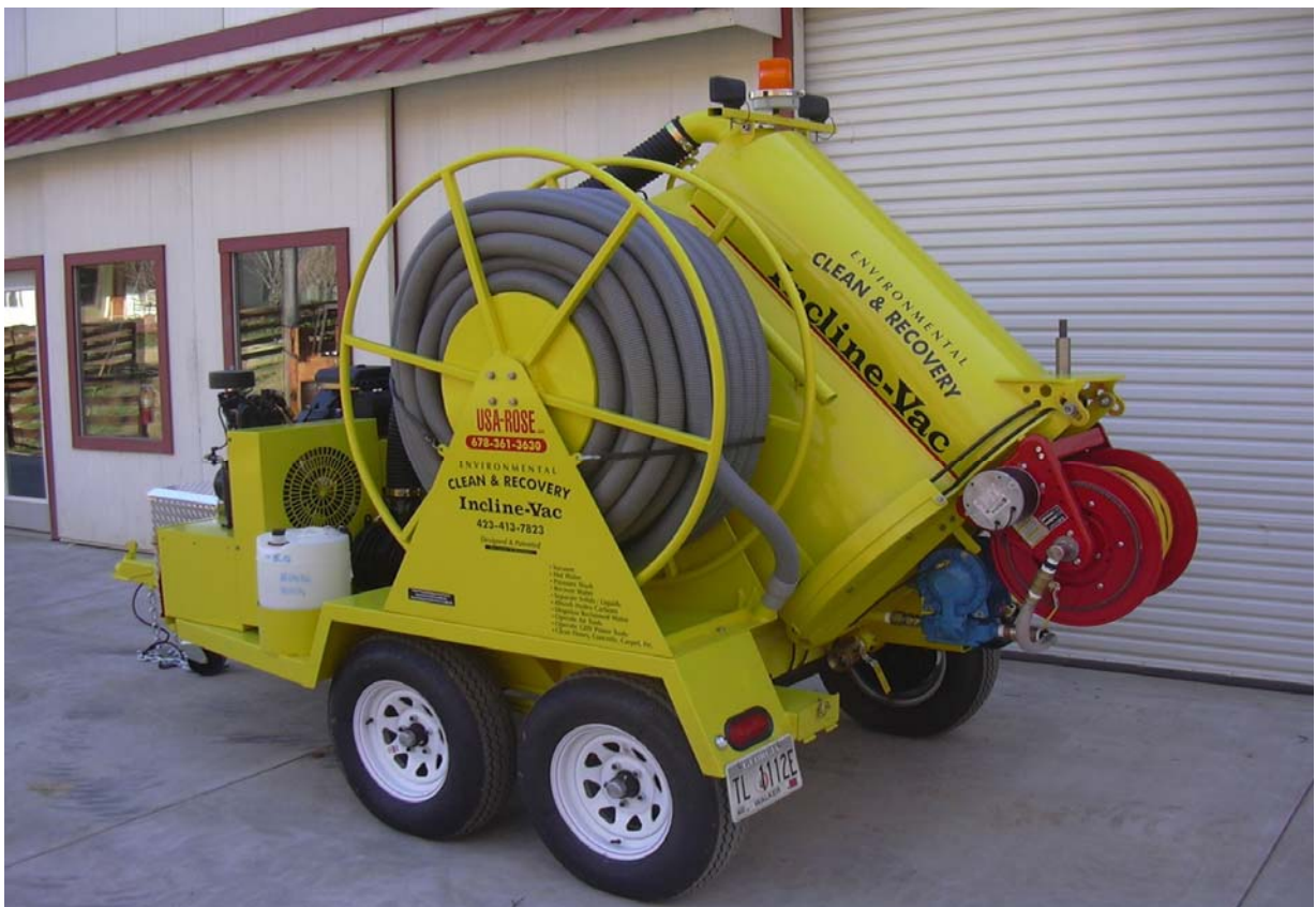
Typical Incline-Vac Hose Reel - picture shows 200' of 2" dia hose or The hose reel holds 100' of 3" dia. vacuum hose
